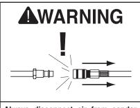
Always disconnect air from sander whenever servicing! During maintenance, a sander connected to air may start accidentally, causing personal injury!
